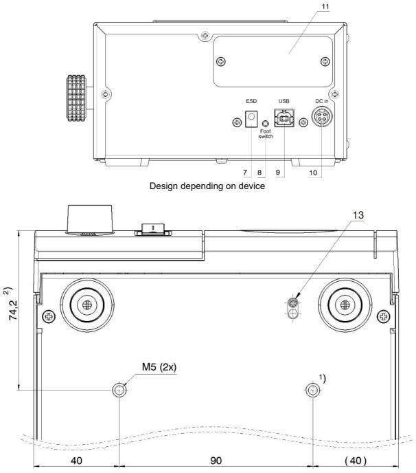
1) max. screw-in depth 7mm measured from outer housing surface 2) measured to vertex of front
